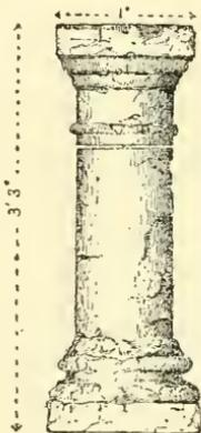
FIG. 4.—Roman Shaft re-used in belfry stage of Saxon Church Tower, Wickham, Berks.
