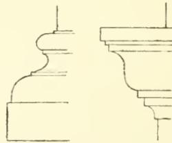
FIGS. 23 and 24.—Base of half-column and impost of main arches, Lorsch.
