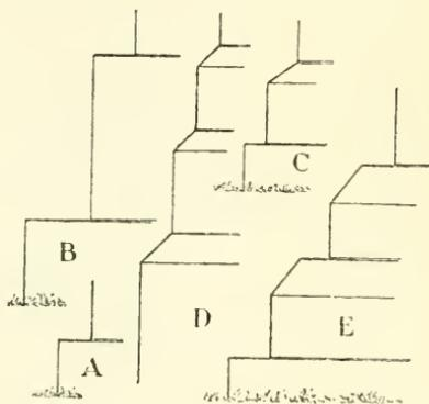
FIG. 31.—Plinths of Anglo-Saxon walls.
