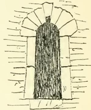
FIG. 43.—Window with sloping jambs, at Brigstock. Do.
