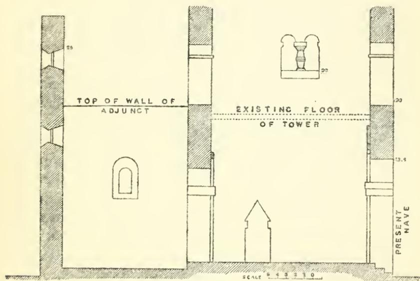
FIG. 130.—Section of tower and western adjunct, Barton-on-Humber.
